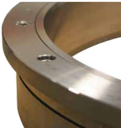
Upgraded upper and lower seats in DeltaValve's top unheading valve combine to improve seal performance and reduce steam consumption. The cartridge-style dynamic seats allow for easy replacement of previous versions. This design includes Inconel coil springs with tight spacing to create even-load distribution, resulting in a consistent seal against the valve gate.
